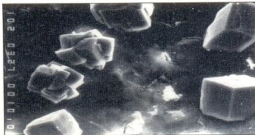
1. An untreated control sample was sheared through at 50 mm below the end surface and the photograph is of the sheared face. Precipitated \text{Ca}(\text{OH})_2 Calcium Hydroxide together with cubic and rhombic particles are visible.
