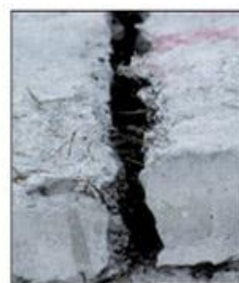
STEEL FIBRE ۵۴.۴% RETENTION OF ENERGY ABSORPTION
